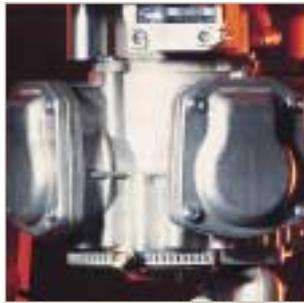
A valve actuated by the crankshaft travels along a linear axis to connect the cylinders successively with the meter inlet and outlet. The valve is mounted between a slide plate built into the meter body and a
